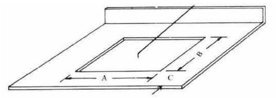
Models 49-26: Minimum horizontal distances from edges of range to adjacent vertical walls above counter level is 2 inches at sides and 3 inches at back. Minimum spacing between adjacent two-burner ranges is 8 inches.
